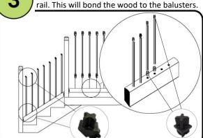
Apply pre-drilled top rail. Attach Cap rail.
