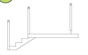
Slide Rail Hanger Bracket over the end of the rail and attach with screws through end of rail. (Hint: Opening of bracket must always be up)
