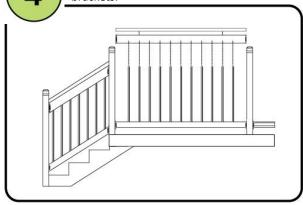
(Note: Optional stair connectors change the baluster to rail connection to a 35-degree exterior stair angle. Simple! Check with the local building department as local building codes and by-laws may apply.)
