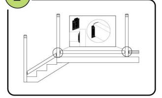
With a high-quality polyurethane construction adhesive, fill all the holes half way. Insert balusters with adaptors into pre-drilled holes in rail. This will bond the wood to the balusters.
