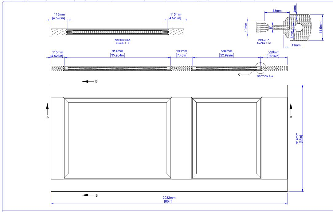
TWO PANEL 45 mm (1 3/4") Two Panel 19 mm Raised SGL-2S Standard VG Ovolo Sticking
