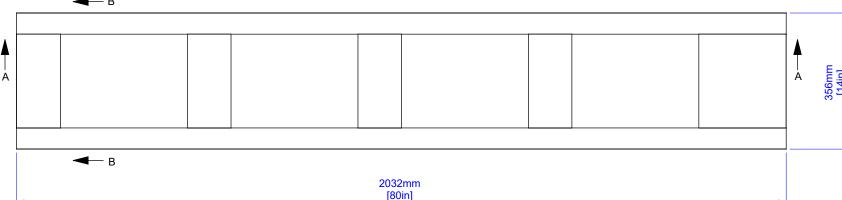
Customer: **Trimming Limits** FLAT PANEL 35mm (1 3/8") Four Flat Panel Horizontal 12mm Standard VG Square Sticking 000 **FSC Wood Statistic** Size in Inch Decimals: Size in Milimeter: **Drawing Code:** Model: 16/09/24 X1 = (18mm) [0.71In]A022378 0719-C 1.38 x 14 x 80 35 x 356 x 2032 1:10 0.017819m<sup>3</sup>X2 = (36mm) [1.42In]MANUFACTURERS OF QUALITY DOORS
