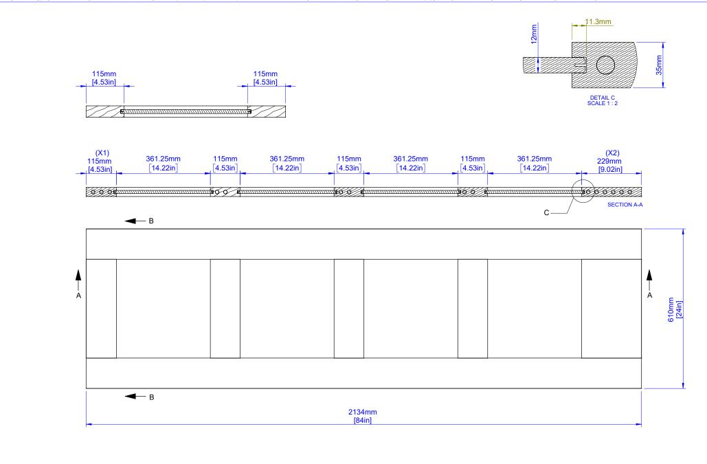
Customer: **Trimming Limits** FLAT PANEL 35mm (1 3/8") Four Flat Panel Horizontal 12mm Standard VG Square Sticking 000 **FSC Wood Statistic** Size in Inch Decimals: Size in Milimeter: **Drawing Code:** Model: 27/01/23 X1 = (18mm) [0.71In]1.38 x 24 x 84 35 x 610 x 2134 A015002 0719-B 1:10  $0.033115m^{3}$ X2 = (36mm) [1.42In]MANUFACTURERS OF QUALITY DOORS
